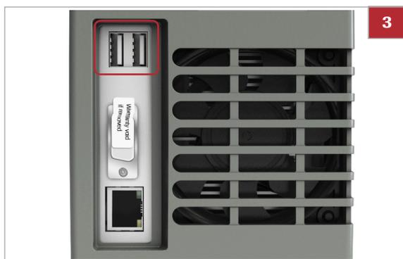
3 Connect the printer to the analyzer.
