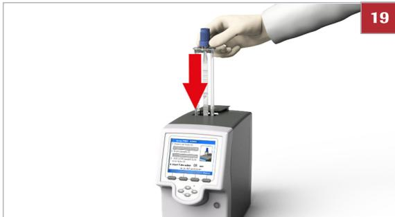
19 Within the time limit for inserting assay tubes, insert the prepared assay tube in the analyzer.
