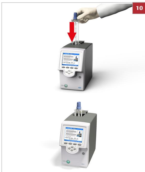
**10** Within the time limit for inserting assay tubes, insert the prepared assay tube in the analyzer.
