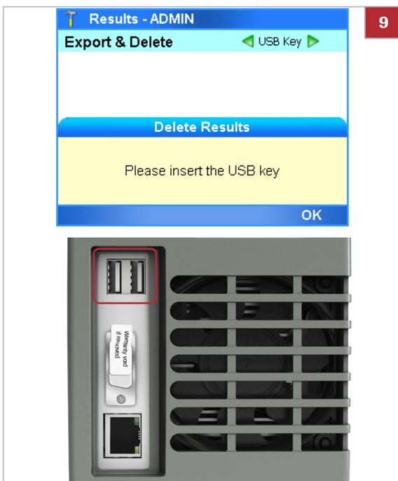
9 If you use a USB key, insert the USB key at the rear of the analyzer. Choose the **OK** button.
