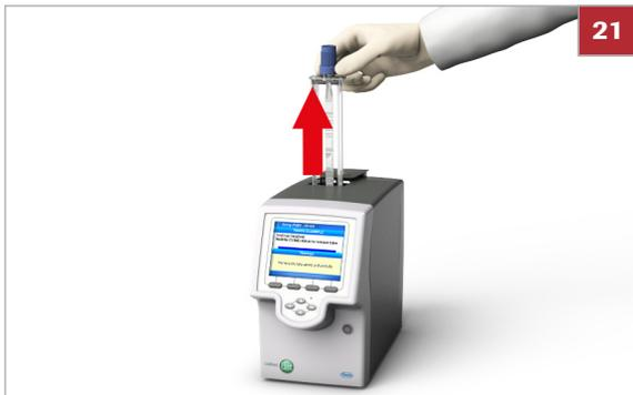
21 When asked to do so, remove the assay tube from the analyzer. Dispose of the assay tube in accordance with the disposal policy of your institution and according to local regulations.
