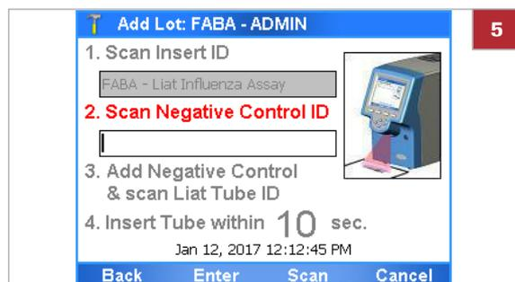
**5** Choose the **Scan** button and place the barcode of the negative control under the barcode reader.
