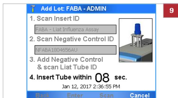
**9** Place the prepared assay tube under the barcode reader.
